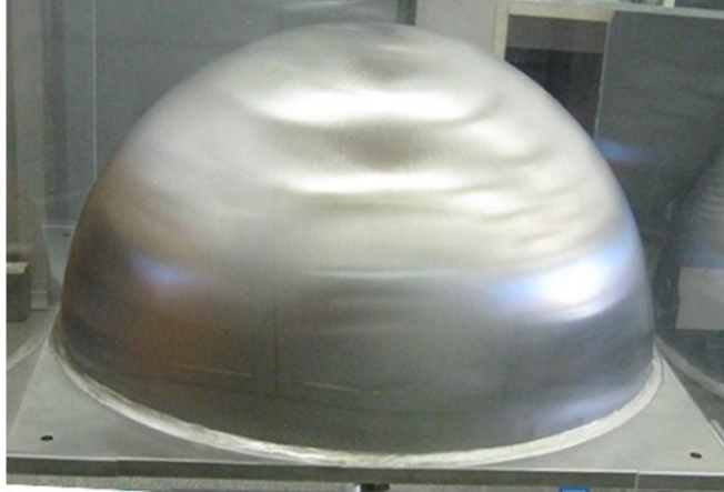
Hemisphere made of stainless steel with a volume V = 50 l
